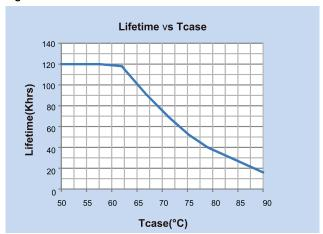
Failure Rate Info based upon MTBF modeling: 90% survivals at end of life @ <=Tc lifetime rating
