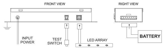
**IMPORTANT:** Do not connect battery until fixture is installed
