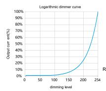
Remarks: The dimming curve can be selected by DALI configuration.
