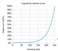
Remarks: The dimming curve can be selected by DALI configuration.
