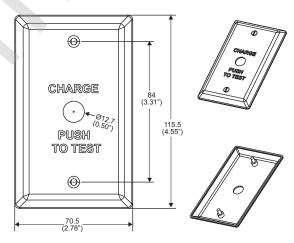
1."Charge push to Test"plate 2. (2) 6-32 x ½"LG mounting screws
